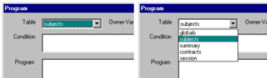
Figure 3.2: In the program dialog it has to be specified in which table the program will run.
